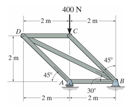
2. Determine the horizontal and vertical components of force which the pin at C exerts on member BC of the frame in figure below.
