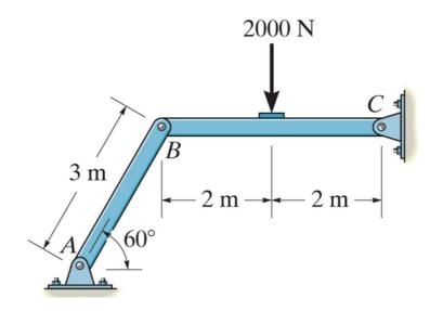
3. The compound beam shown in figure below is pin connected at B. determine the components of reaction at its supports. Neglect its weight and thickness.
