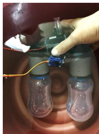
Figure 1: The water sampler being tested in a basin at vertical position
