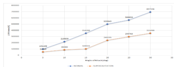
Figure 2: Lift Characteristics of Fin Stabilizer
