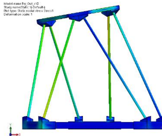
Figure 1: Result simulation on stress of motion platform when tilt left-side 10°
