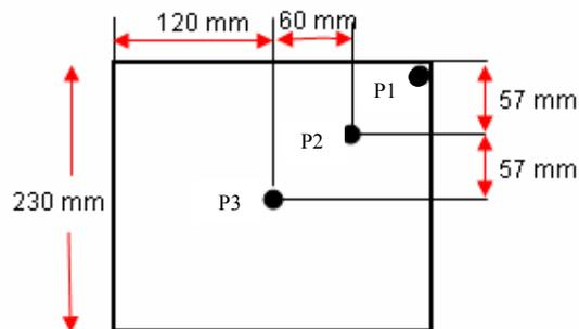
Figure 1 : Layout of accelerometer location on the plate
