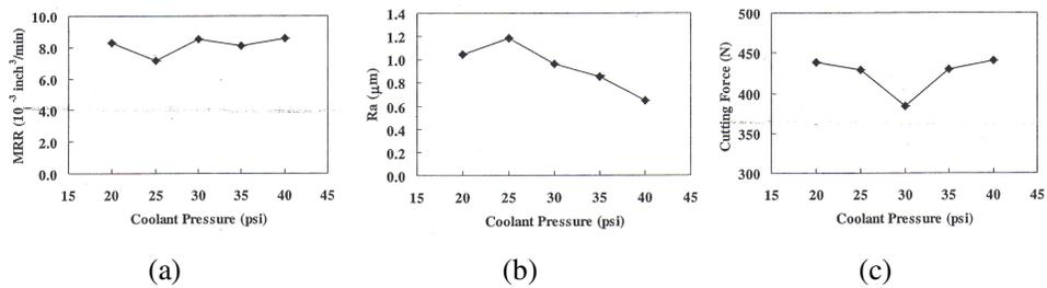
Figure 11: Effect of coolant on RUM of alumina [16]
