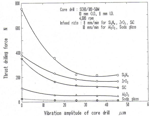
Figure 7: Effect of vibration amplitude on cutting force [2]
