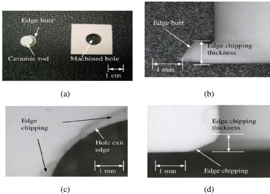
Figure 14: Edge chipping induced by RUM (a) Two parts resulting from RUM
