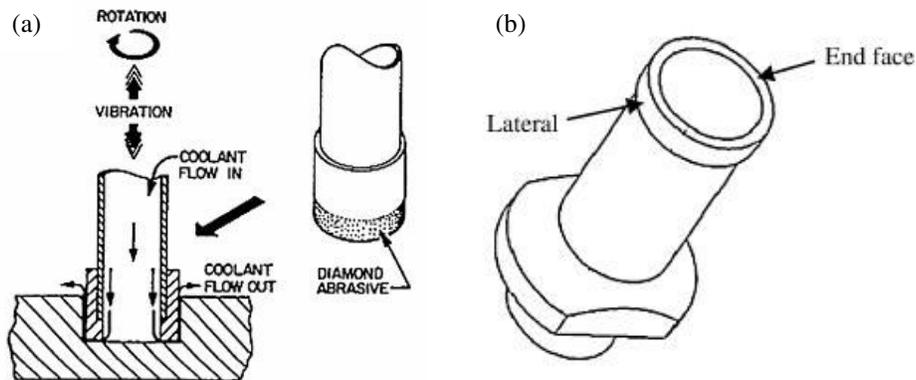
Figure 2: Schematic illustration of rotary ultrasonic machining
