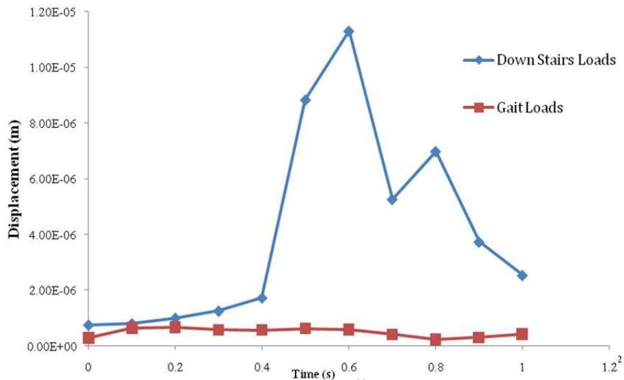
Figure 4: Deflection data between Gait Loads and Down Stairs loads
