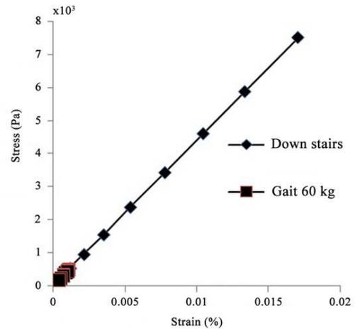
Figure 6: Down stairs Loadings and Gait Loadings for bodyweight 60kg
