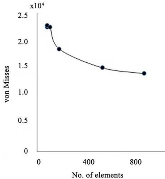
Figure 3: Plotted graph of von-Misses against number of elements, indicated in the region of 700,000 to 800,000 considered as optimum numbers
