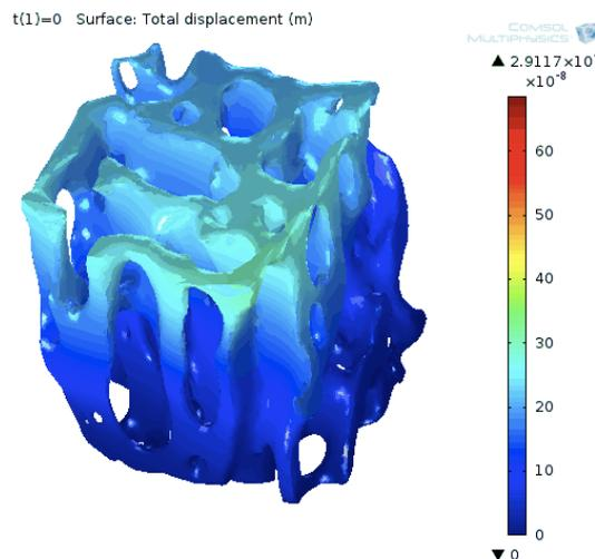
Figure 8: Total displacement of normal walking with 60 kg bodyweight load
