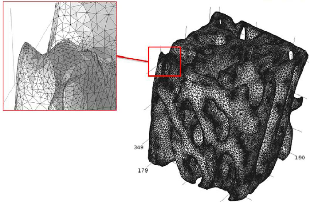
Figure 1: Meshed specimen with 774,996 numbers of elements created to satisfy finding in converged region.
