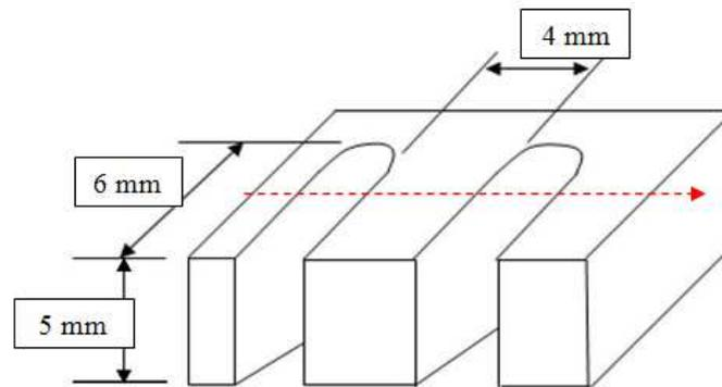
**Figure 1** The diagram of cutting direction on the work material.
