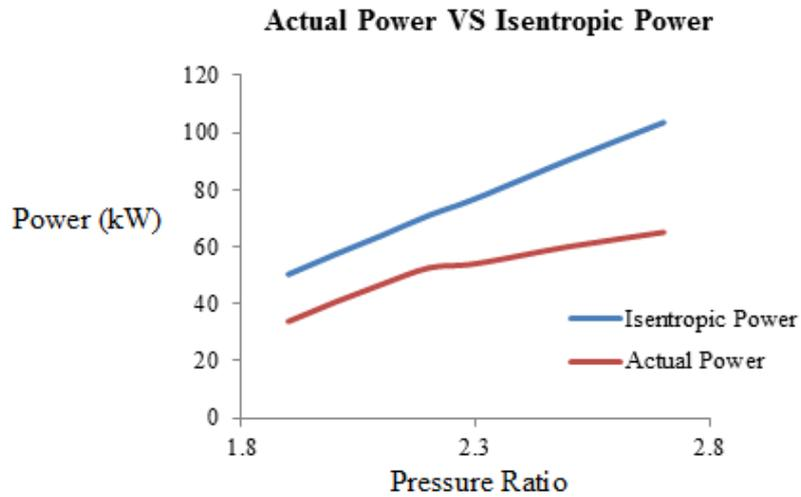
Figure 19: Deviation of turbine actual power with isentropic power
