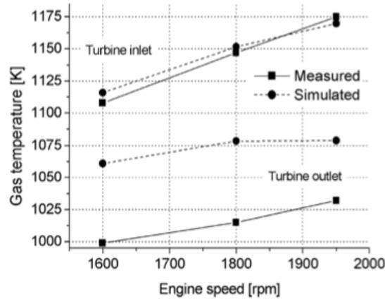
Figure 4 : Measured and simulated turbine inlet/outlet temperature [2]
