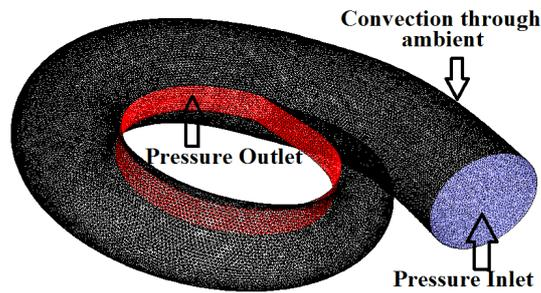
Figure 16: Types of boundary condition for simulation
