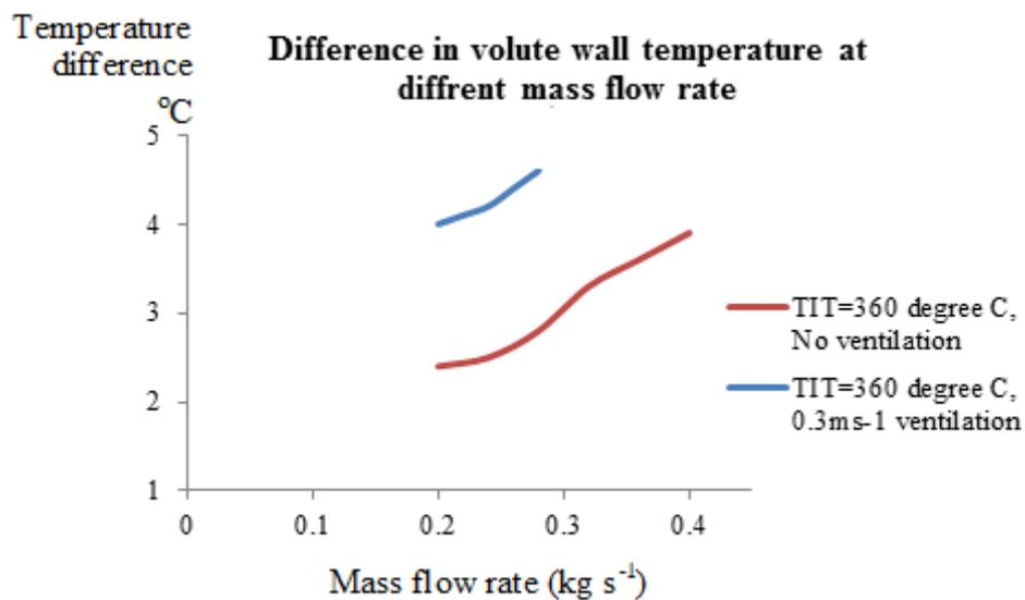
Figure 24 : Difference of temperature between inner and outer turbine's volute wall [3]
