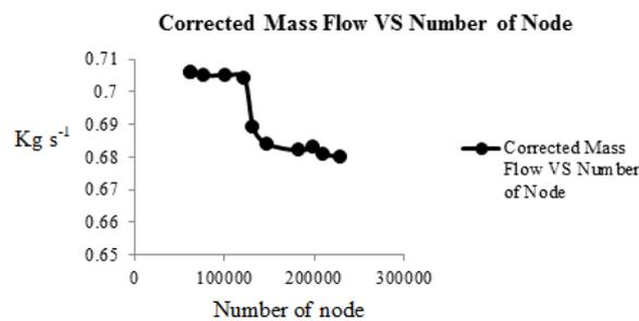
Figure 14: Grid independent study of corrected mass flow
