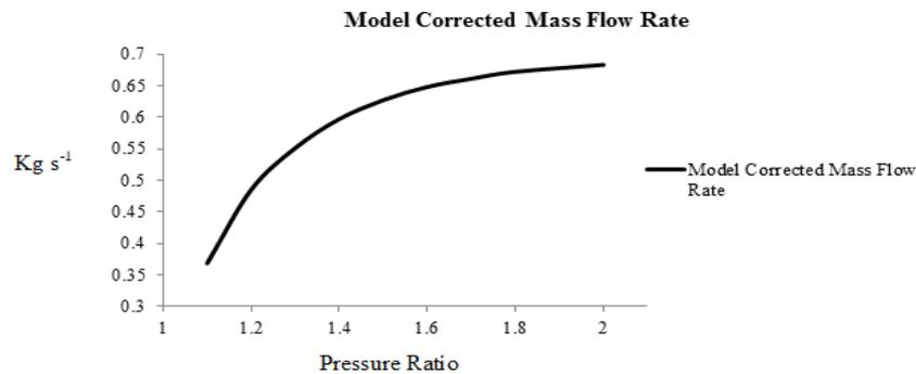
Figure 17: Simulation of corrected mass flow rate
