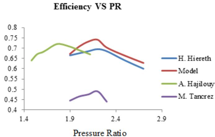
Figure 21: Comparison of adiabatic efficiency
