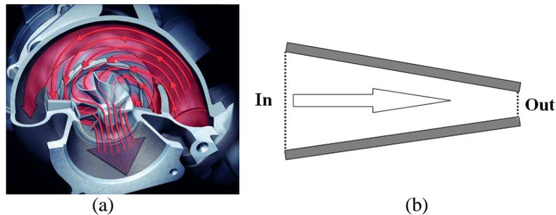
Figure 5: (a) Actual turbine area, (b) Simplified model of turbine volute (Converging nozzle)
