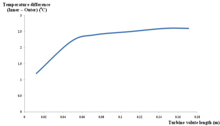
Figure 11: Temperature difference between inner and outer of turbine volute wall
