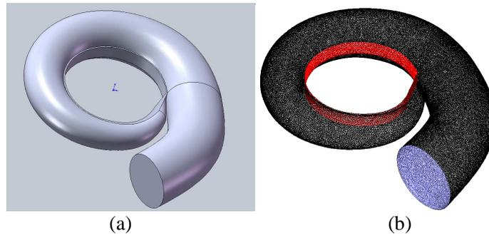
Figure 13: (a) Turbine volute model in SOLIDWORKS, (b) Meshed model of turbine volute in GAMBIT
