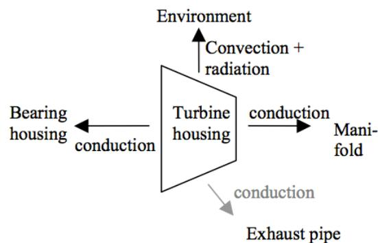
Figure 1 : Heat losses around turbine volute [3]
