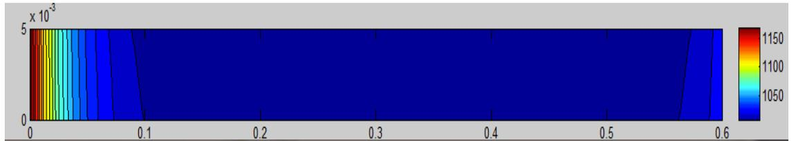
Figure 10 : Temperature contour from 2-D analysis
