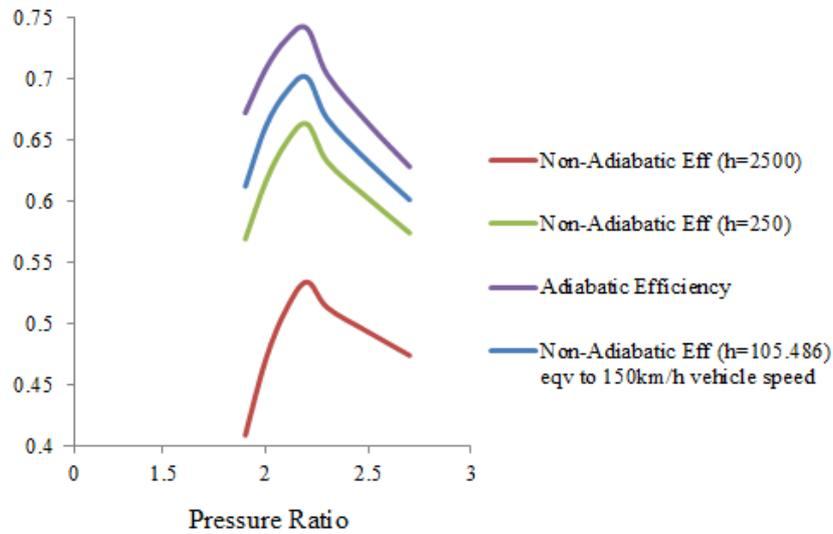
Figure 25: Comparison of efficiency for different cases
