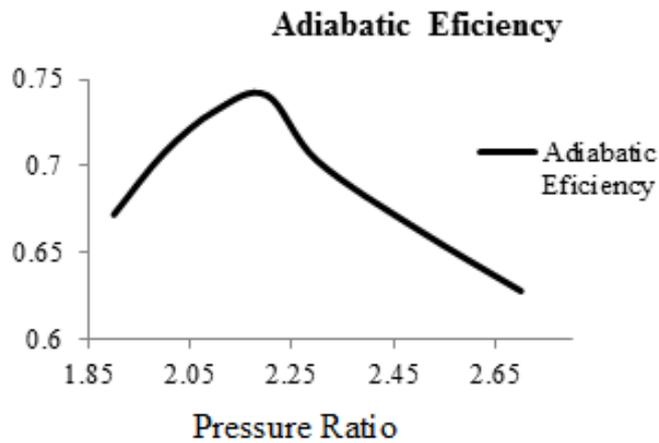
Figure 20: Turbine's adiabatic efficiency
