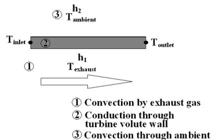
Figure 9: Boundary condition for two-dimensional analysis
