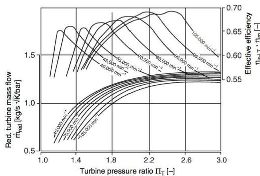
Figure 3 : Turbine map with mass flow parameter and turbine efficiency [10]
