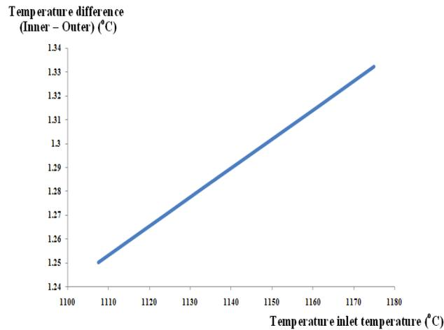
Figure 8: Temperature difference from one-dimensional analysis
