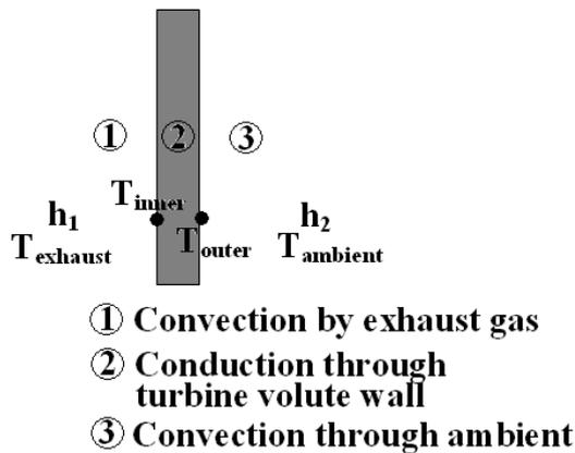
Figure 6: Boundary condition at volute wall for 1-D analysis
