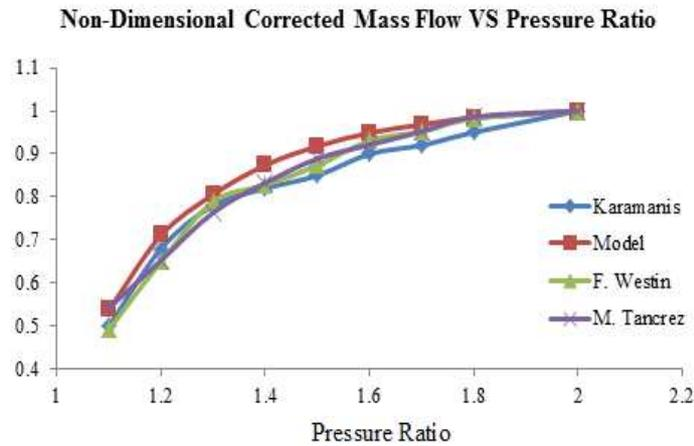
Figure 18: Comparison of non-dimensional corrected mass flow rate
