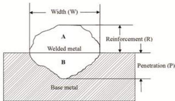
Figure 1: Weld bead geometry
