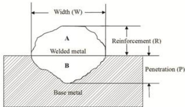
Figure 1: Weld bead geometry
