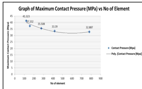
Figure 8: Graph of Maximum Contact Pressure (Mpa) against No of Element.
