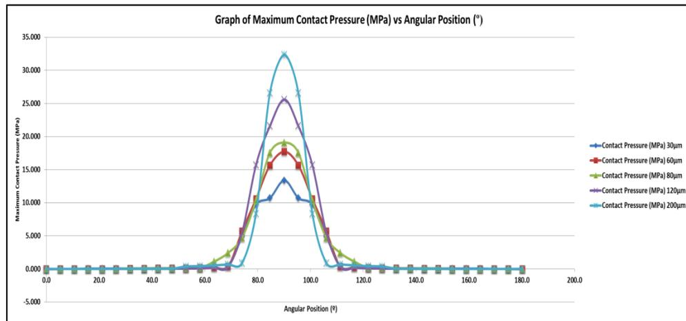
Figure 10: Graph of Maximum Contact Pressure (MPa) versus Angular Position (°) (Lubrication Contact) – Constant Femoral Head Size
