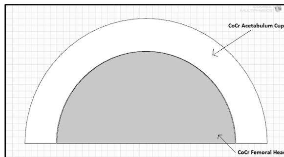
Figure 3: The Whole Structure of Hip Joint Implant Model
