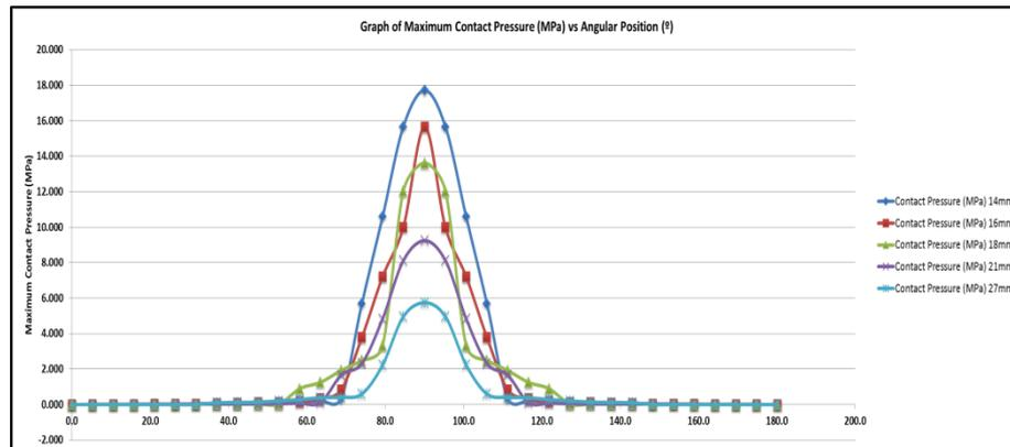
Figure 13: Graph of Maximum Contact Pressure (MPa) versus Angular Position (°) (Lubrication Contact) – Constant Radial Clearance
