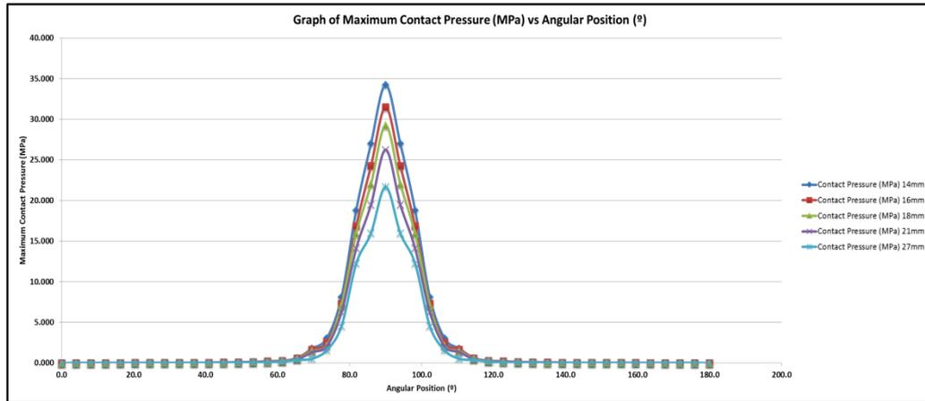
Figure 12: Graph of Maximum Contact Pressure (MPa) versus Angular Position (°) (Dry Contact) – Constant Radial Clearance
