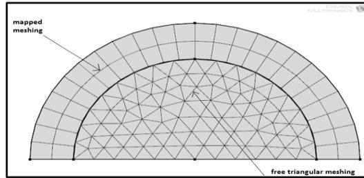
Figure 5: Mesh Shape of the Hip Implants Model
