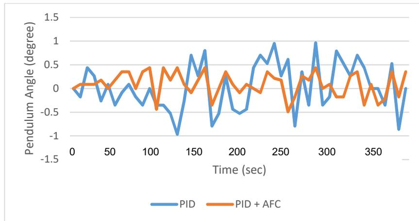
**Figure 17:** Comparison of pendulum angle responses between the PID and PID+AFC controllers
