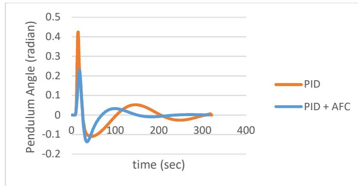
**Figure 12:** Comparison of pendulum angle response between the two controllers
