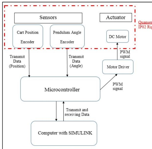
Figure 14: Schematic diagram of the inverted pendulum experimental rig
