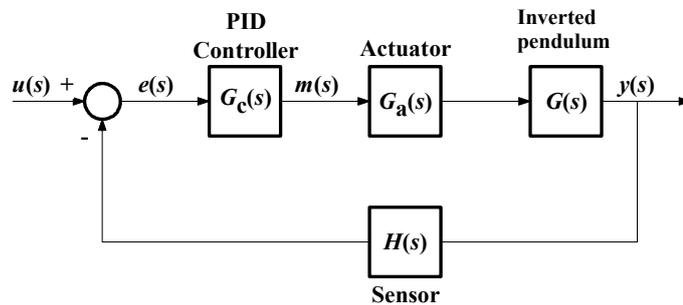
Figure 2: PID control applied to the inverted pendulum
