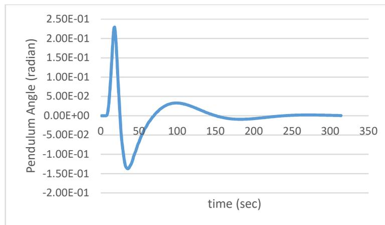
**Figure 10:** PID+AFC pendulum angle response
