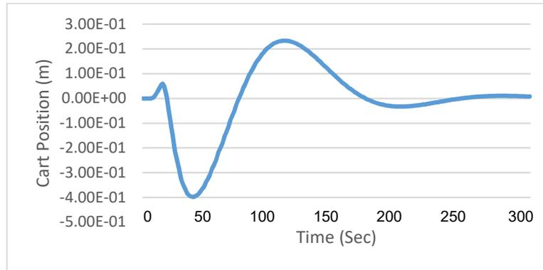
**Figure 9:** PID+AFC controller cart position response
