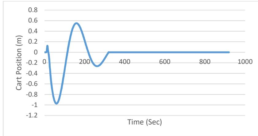
**Figure 6:** PID controller cart position response
