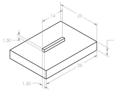
**Figure 2:** Geometry of the microchannel mold E (in mm)
