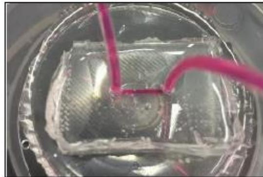
**Figure 4:** PDMS microchannel during functional testing
