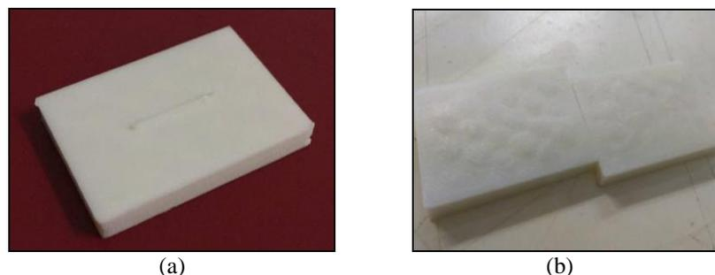
**Figure 3:** 3D printed microchannels produced using different two 3D printers: (a) *ANYCUBIC DIY Kossel* (b) *Double Nozzle 3D Printer Creator Pro*
