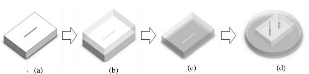
**Figure 1:** Fabrication of the PDMS microchannel from 3D printed mold
