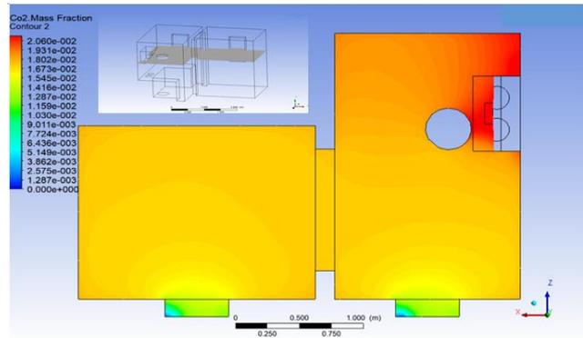
**Figure 4:** Distribution of CO<sub>2</sub> mass fraction for Case 1 (top view)
