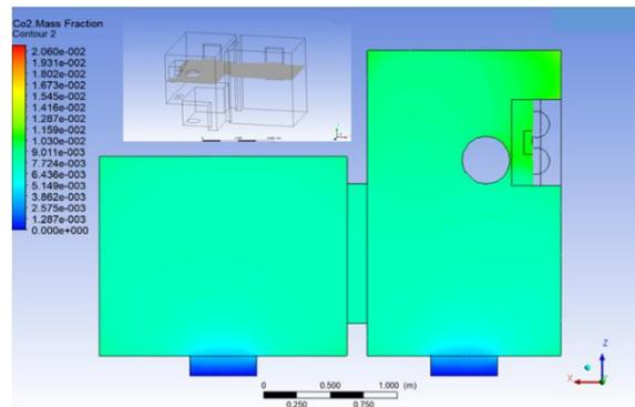
**Figure 5:** Distribution of CO<sub>2</sub> mass fraction for Case 2 (top view)
