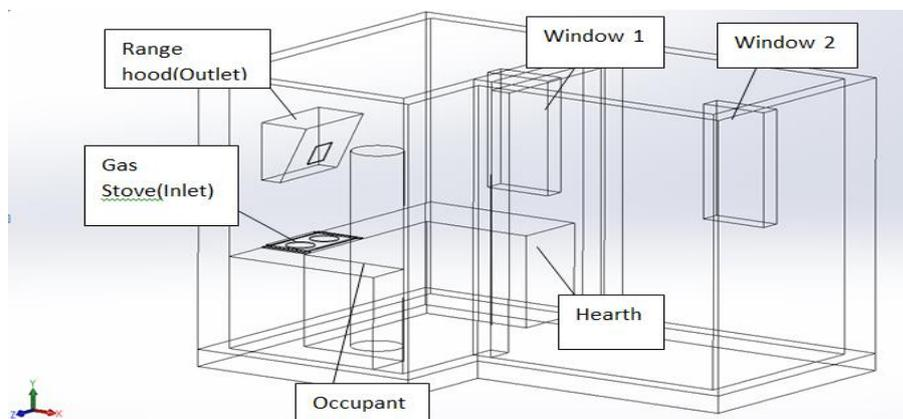
**Figure 1:** CFD model of a kitchen
