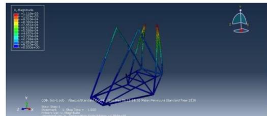
Figure 24: Deflection of main frame for Case 1
