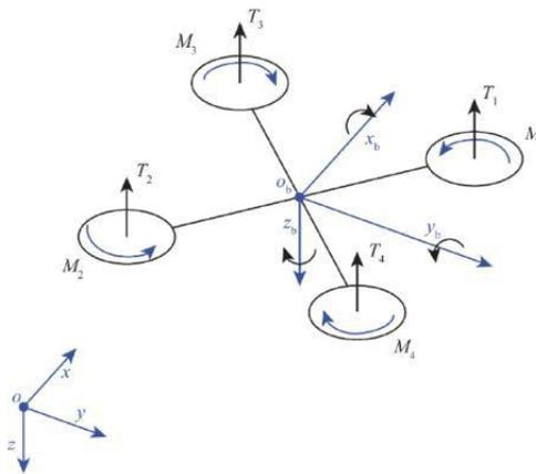
**Figure 1:** Quadrotor dynamics [5]
