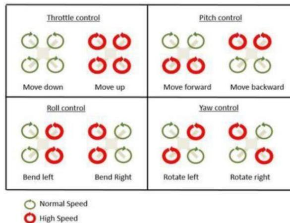
**Figure 2:** Alternative working principle of a quadrotor [6]
