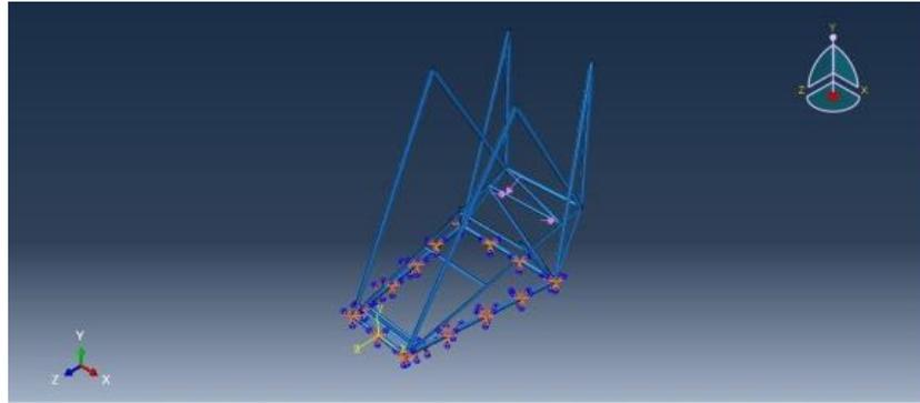
**Figure 11:** Strength analysis of the seat support
