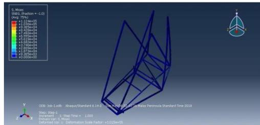
**Figure 25:** Stress distribution of main frame for Case 1
