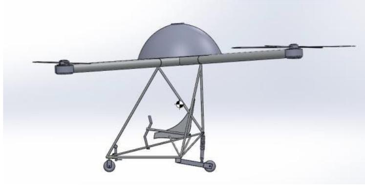
**Figure 9:** The center of gravity of the quadcopter
