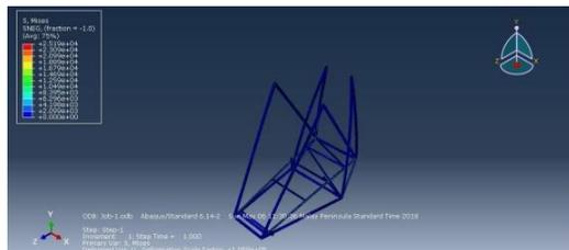
Figure 23: Stress distribution of main frame for Case 1
