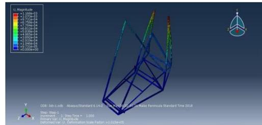
**Figure 26:** Deflection of main frame for Case 1
