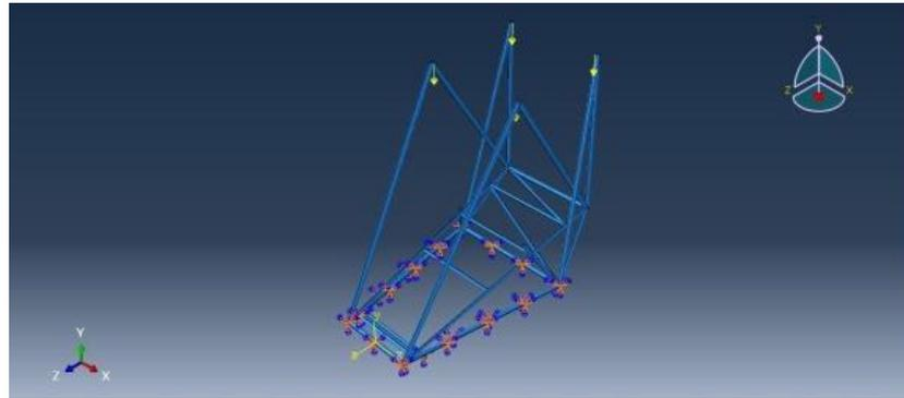
**Figure 12:** Analysis of buckling of column
