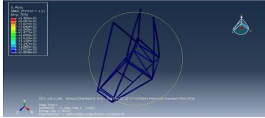
Figure 19: Stress distribution of the main frame
