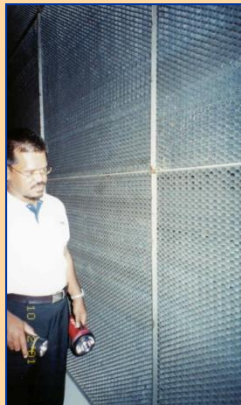
Settling Chamber • Heat Exchanger • Honeycomb • 3 Screens
