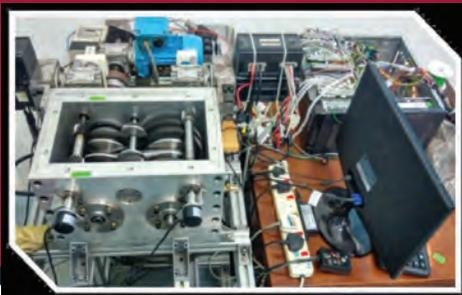
**Design and development of an electro-mechanical CVT for automotive applications**
